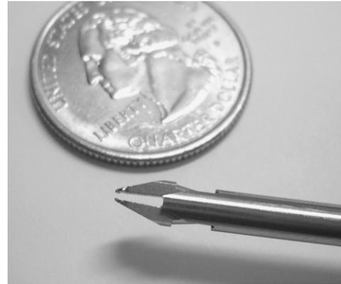
**FIGURE 5.** Photograph showing new fixation sleeve without a J-slot, for less cumbersome welding and easy release.
